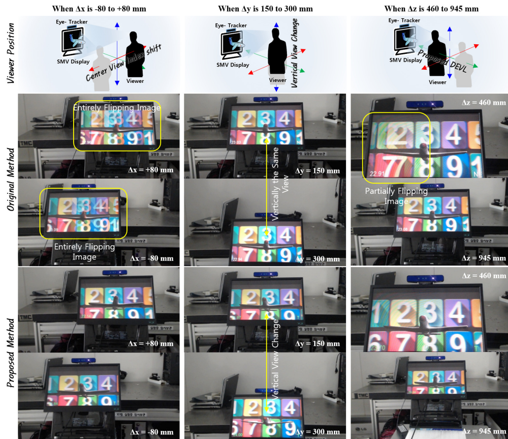
Fig. 12. An application of the proposed method toward viewing-lobe-free and visually comfort 3-D perception. Our prototype of head-tracked SMV display, combined with the conventional head-tracking technology, allows a viewer to see natural 3-D contents at any positions in the xyz-direction, and it works in 22–24 fps including the function of vertical view changes in the practical environment (see Visualization 3 , Visualization 4 , Visualization 5 , and Visualization 6 ).
